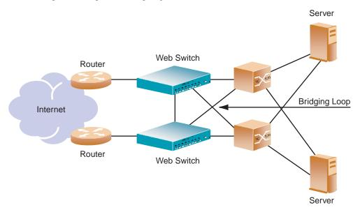
Figure 11-11 Loops in Active-Active Configuration
